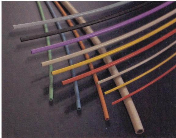
PEEK (polyetheretherketone) polymer tubing is biocompatible, chemically inert to most solvents, and can be used to replace stainless steel tubing in most liquid analytical systems. Unlike stainless steel and titanium tubing, PEEK tubing is flexible and can be easily cut to desired lengths. PEEK tubing can be used with stainless steel or polymer fittings.
