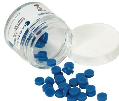
The Economy **diskobolus™** Blue septa are designed for non-demanding, routine applications. They are easy to penetrate. These septa can be used up to 250°C and are suitable for 90% of all GC analysis. Made from silicone. The package is for 100 pieces.
