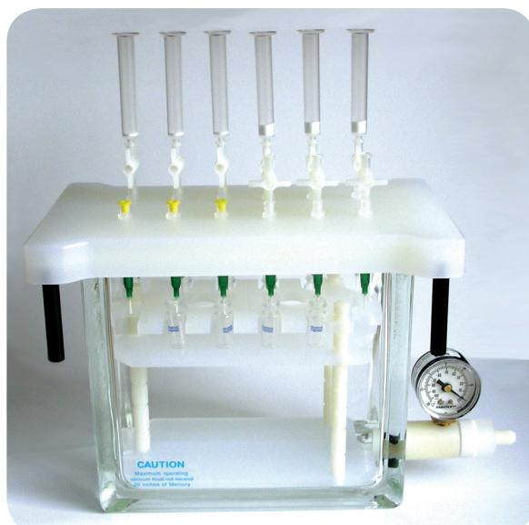
Teknokroma vacuum manifolds simplify SPE sample processing. These manifolds permit consistent extraction and filtration results. Analyst can save time, since these manifolds allow simultaneous multiple sample processing.
