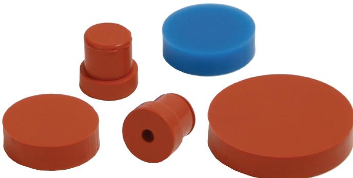
Septum is the most general source of contaminants in the injection port. The baseline noise or the appearance of ghost peaks in the chromatogram can be a consequence of the septum bleed or of the samples of former injections that have been adsorbed on the septum surface.
