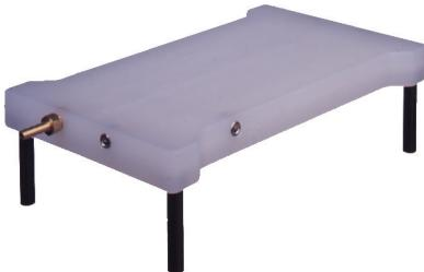
Drying attachments are available for the 12 and 24 port manifolds, which will direct the flow of air or nitrogen into the collection vessels to concentrate eluants, prior to further analysis.
