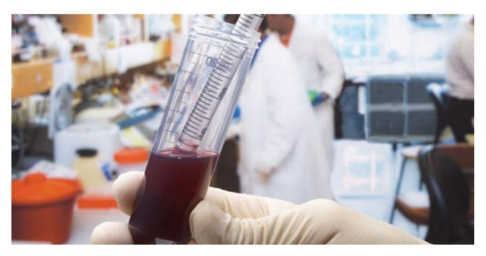
SuperClear™ tubes are made from a unique non-cytotoxic medical grade resin that is clear and very durable, making it possible to spin these tubes at 20,000g for 50ml tubes and 17,000g for 15ml tubes.
