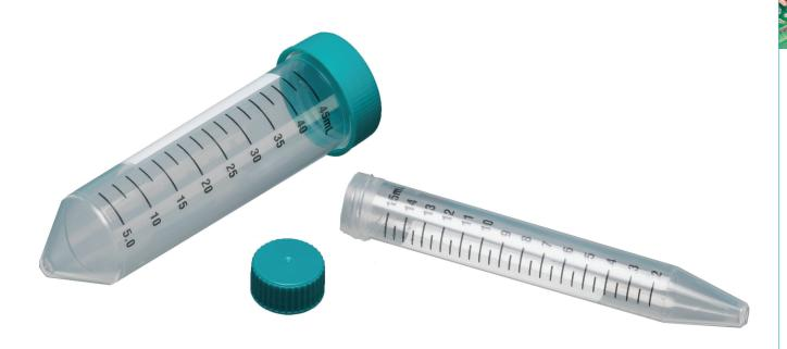
The 50ml tube is available in a free-standing (skirted) format, which allows it to stand upright without the need for a rack. It is ideal for transporting samples since it is lab certified to the IATA 95kPa standard.
