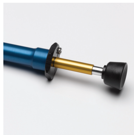
3-000-105 set to dispense 1 \mu l with largest spacer
