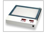
gels simultaneously. The unit's microprocessor controls temperature and time, each parameter being displayed on its own LED display. The gels are heated from the base plate while the vacuum removes the moisture from below to dry the gel homogeneously. These dryers feature optimal sealing using a silicone rubber cover and supporting mask.
