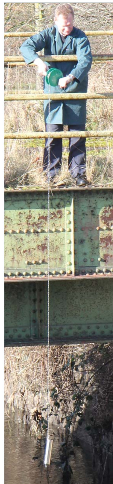
Liquid flows in when the sampler hits the bottom
