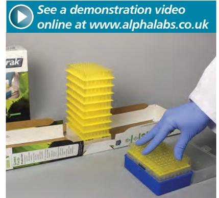
3. Push down on transfer top to release refill plate. Return transfer top to **Fastrak**® refill stack and close.
