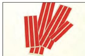
Loading Guides allow easy well identification and sample loading.
