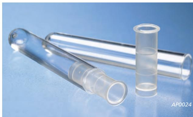
Polypropylene tube insert to convert the volume of a 12mm diameter tube to 1.5ml or 3.0ml.
