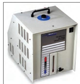
The room temperature vapour trap acts as a pump by condensing the hot vapours from the gel dryer and trapping them from the rest of the systems. The high efficiency diaphragm pump, delivers a powerful, non-fluctuating vacuum for fast, smooth drying. GelMaster™ is so efficient it can be connected to 3 gel dryers simultaneously. 10-15 gels can be dried before the trap needs to be drained. The GelMaster™ trapping medium can be used repeatedly.
