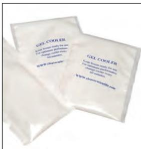
A simple to use cooling pack system ensures enhanced resolution without costly and time-consuming additional equipment. No chiller, tap or obstructing connecting leads are required. The cooling pack is simply pre-chilled in a freezer and placed in the gel tank. Additionally, the use of cooling packs reduces buffer volume.
