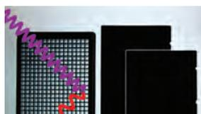
For top-reading fluorescence applications, apply the black sealing film to the base of clear-bottomed plates. For bottom-reading fluorescence, use the black sealing film as a top seal.
