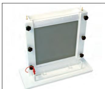
Resolution is enhanced by using an aluminium heat sink plate, which is essential for even sample migration.
