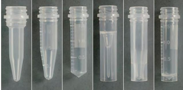
APEX® Screw-Cap Microcentrifuge Tubes are ideal for sample collection, processing and storage. Manufactured from virgin polypropylene, this range of tubes has low-binding properties and is certified free from RNase, DNase, human DNA and PCR inhibitors. Both cap and tube are produced from the same material and share expansion coefficients to provide uniform rates of expansion and contraction in response to temperature change, offering a high quality leak-resistant design.
