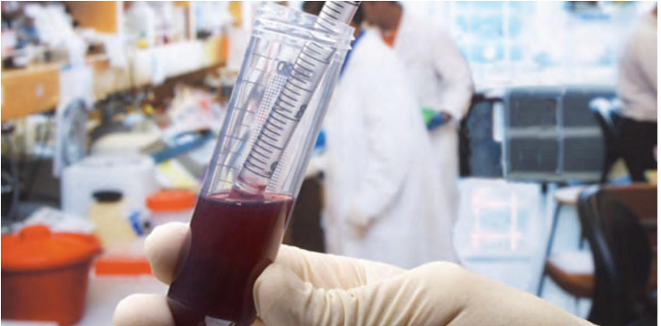
SuperClear™ tubes are made from a unique non-cytotoxic medical grade resin that is clear and very durable, making it possible to spin these tubes at 20,000g for 50ml tubes and 17,000g for 15ml tubes.
