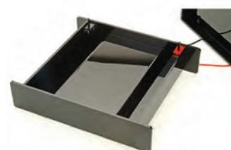
Each tank's robust construction from ebony acrylic ensures that cells remain free of exposure to background light and DNA damage during electrophoresis, while a cooled central platform provides a convenient surface for slide preparation and control of slide temperature during the assay. Following electrophoresis DNA damage may be measured using Comet Assay scoring software.
