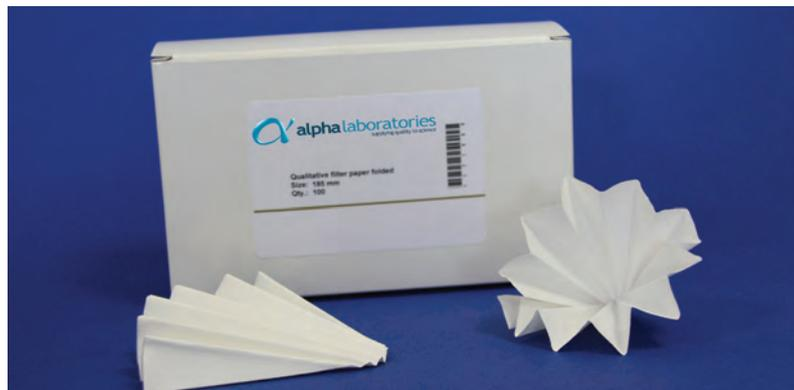
**Grade 601 - Medium filtration velocity filter paper used for analytical work in laboratories. Equivalent to Whatman® No.1 and Schleicher and Schuell® 595**
