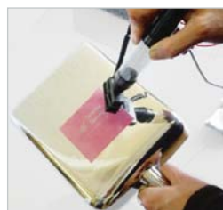
3. Place the Etching Mask and apply the etching fluid using the Electrolyte Applicator
